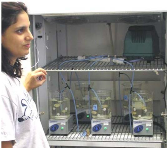
**Monica Torres-Ruiz demonstrates the successful design for the flow-simulating caddisfly beakers with stir plates and an incubator.**
