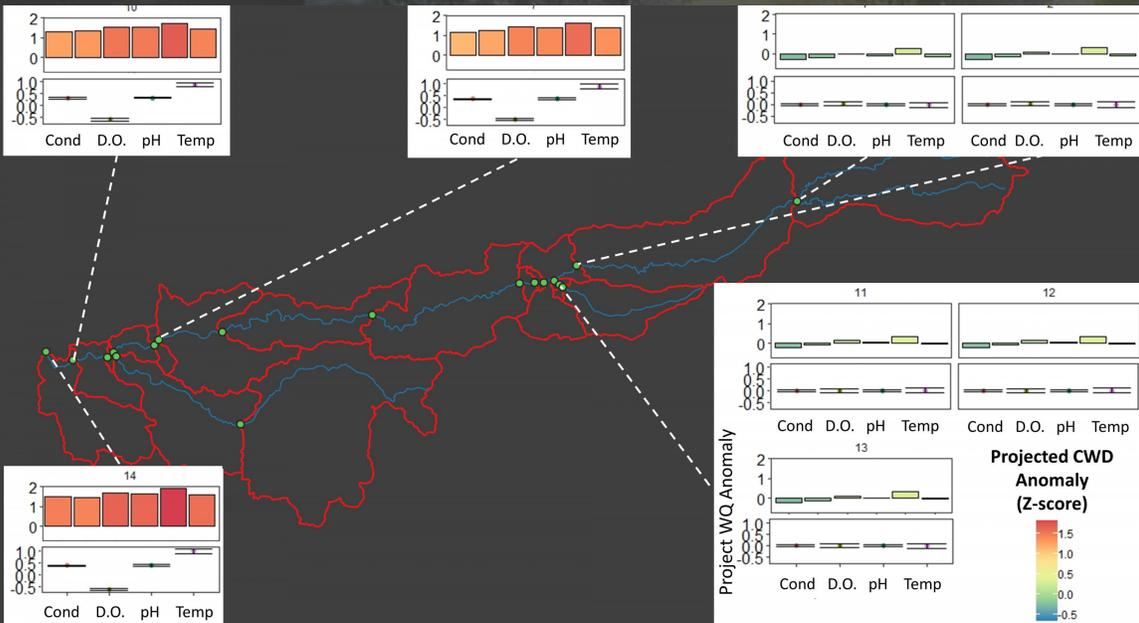
Figure 2 (left): Projected aridity anomaly (red bars) and resulting water quality at subset of sampling locations (green dots) in the Deer Creek watershed in the Sierra Nevada mountains by 2099. Projected aridity drawn from 6 global circulation models that best represent California. Bars that are taller and more red = greater future aridity. Blue bars represent declining future aridity.
